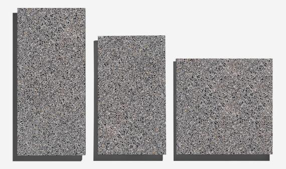
TP-PANELS are made of resin cement and selected aggregates cast onto corrugated aluminium sheets. Stain proof, UV stable and suitable for both indoor and outdoor use, they are 50 percent lighter and significantly stronger than conventional stone and terrazzo slabs. The panels can be used as structural elements thanks to connection pieces set within the material and positioned at will. TP-PANELS are entirely cast, cut and polished by hand in Europe by skilled craftsmen.
